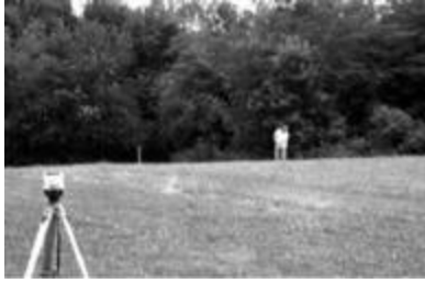
Figure 4. Contour is being marked with grade stakes within the distribution area.
